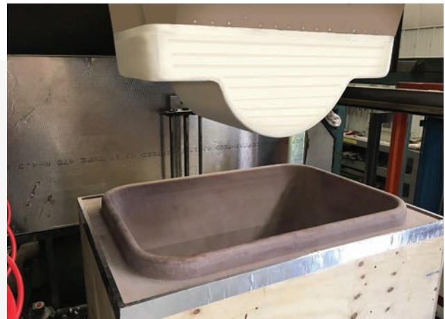
Full Syntactic Plug Assist entering the mold.
