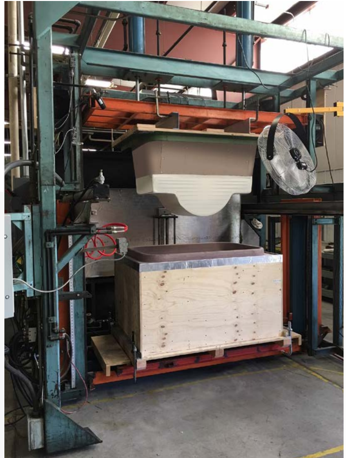
SAYtooling Mold & Plug Assist setup in deep draw forming machine.
