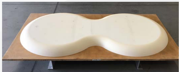
CNC machined mold produced from a HYTAC LPX cast block supplied by CMT Materials
